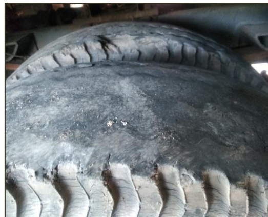
Picture 4 : Poor tyre condition, Bahour fire engine
