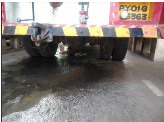
Picture 3 : Intense water leakage, Karaikal fire engine
